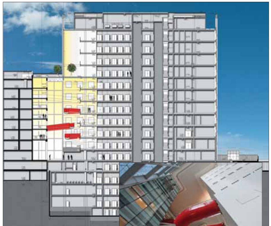
The concept of connecting the old and the new resulted in the design of a connecting atrium with dramatic red bridges.
